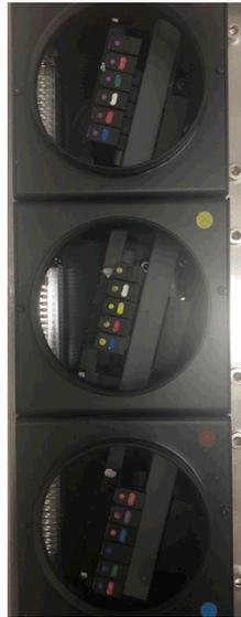
The standard position of the optical filters in the Cytoflex S with **(A)** and without **(B)** the WDM caps.
